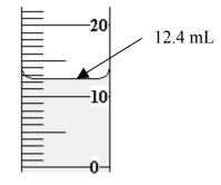
2) Determine the volume of the liquids in the following cylinders:
